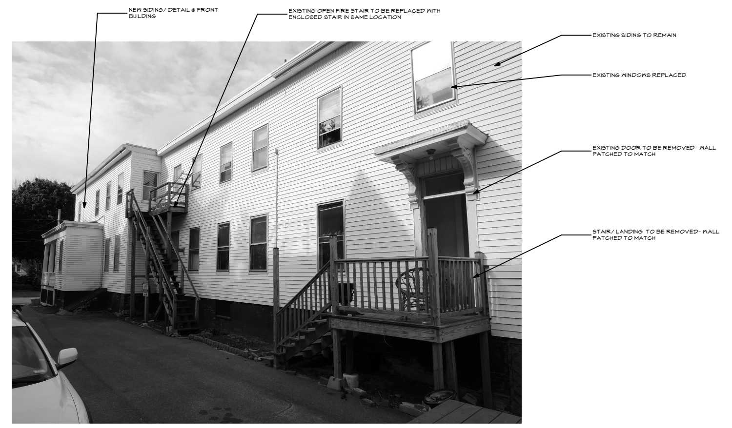
EXISTING DRIVEWAY ELEVATION
