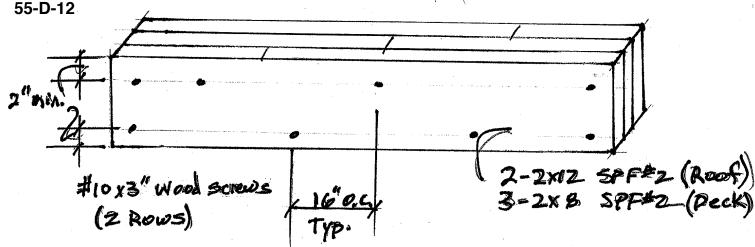
Beam Assembly Detail (U.T.S.) Stagger Splice
