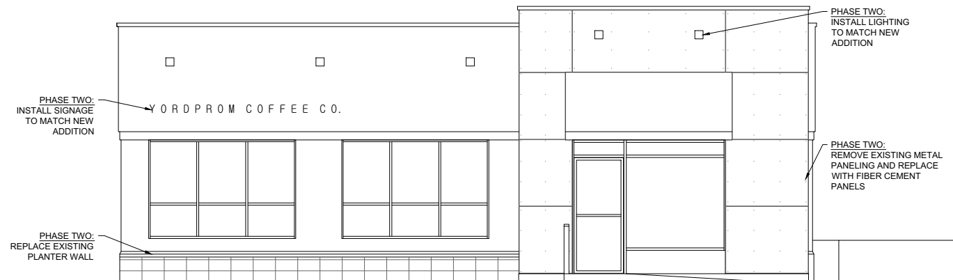
13 NORTH ELEVATION - EXISTING BUILDING PHASE TWO 1/4" = 1'-0"
