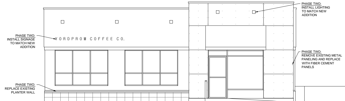
13 NORTH ELEVATION - EXISTING BUILDING PHASE TWO 1/4" = 1'-0"
