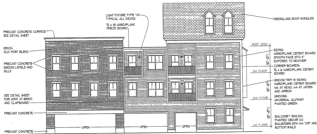
1 CONGRESS ST. FACADE Scale 1/8" = 1'-0" MATERIALS SHOWN ARE TYPICAL FOR ALL FOUR ELEVATIONS. SEE TYPICAL DETAILS ON SHEET 8 OF 8
