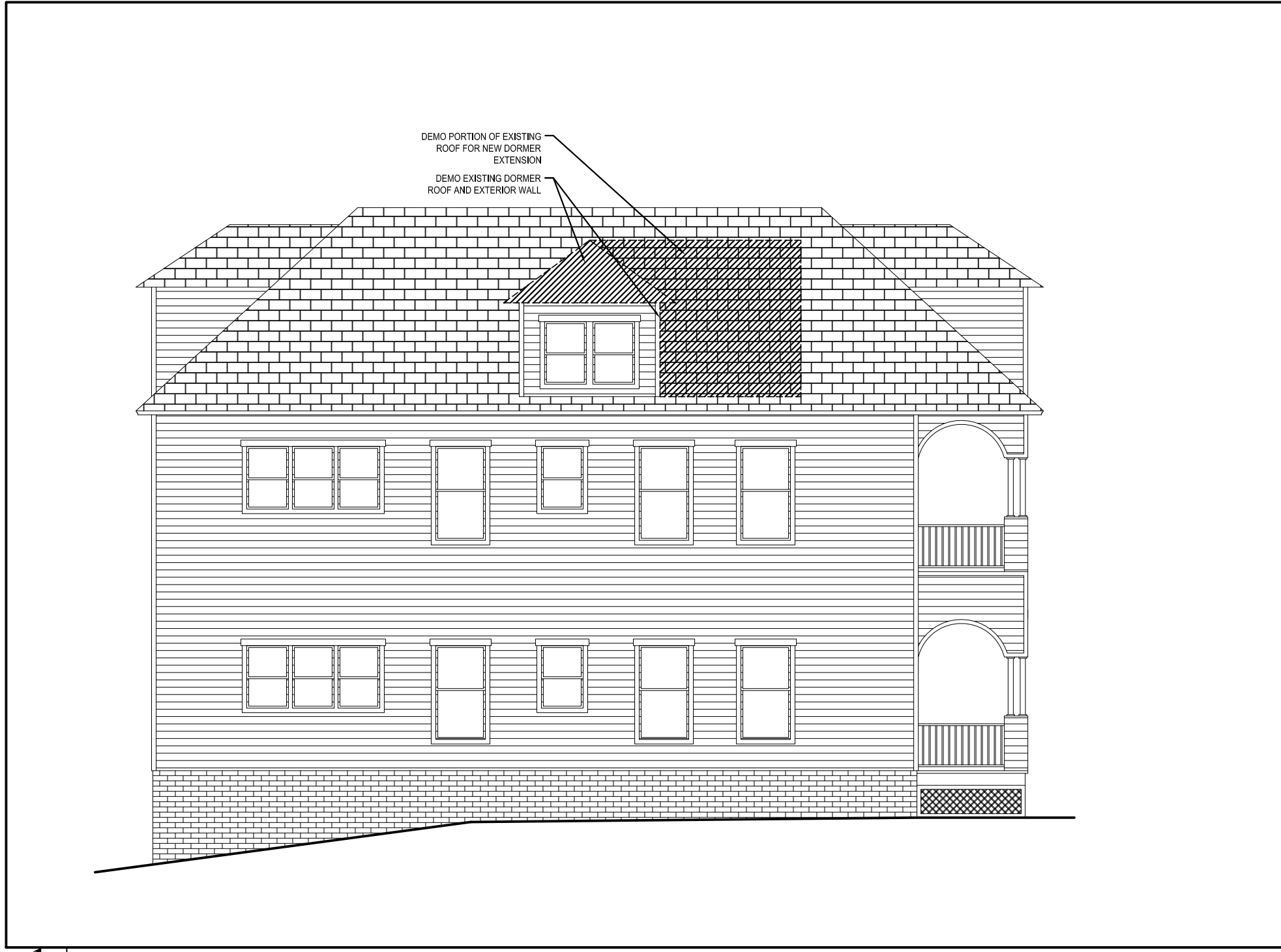
1 EXISTING /DEMO BUILDING ELEVATION SCALE: 1/8"=1'-0"
