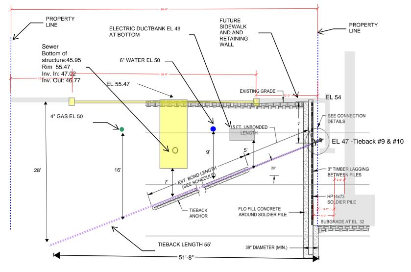
THESE PLANS DETAIL THE TEMPORARY EXCAVATION SUPPORT SYSTEM TO BE INSTALLED AT THE SOUTHWEST THESE PLANS DETAIL THE LEMPORARY EXCAVATION SUPPORT SYSTEM TO BE INSTILLED AT THE SOUTHWEST OCCURRED OF THE NEW CONSIGNES STREET BUILDINGST THE MAINE MEDICAL CENTER IN PORTLAND, MAINE. THE EXCAVATION SUPPORT SYSTEM HAS BEEN DESIGNED FOR A MAXIMUM VERTICAL SURCHARGE OF 300 PSF APPLIED AT THE TOP OF THE SUPPORT WALL.
