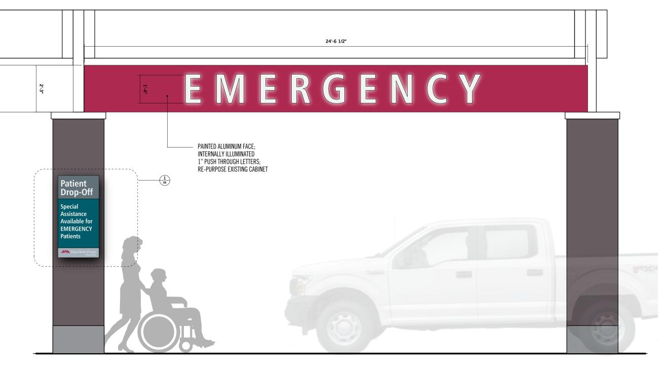
Elevation: ST.2b Canopy ID scale: 1/2" = 1' - 0"
