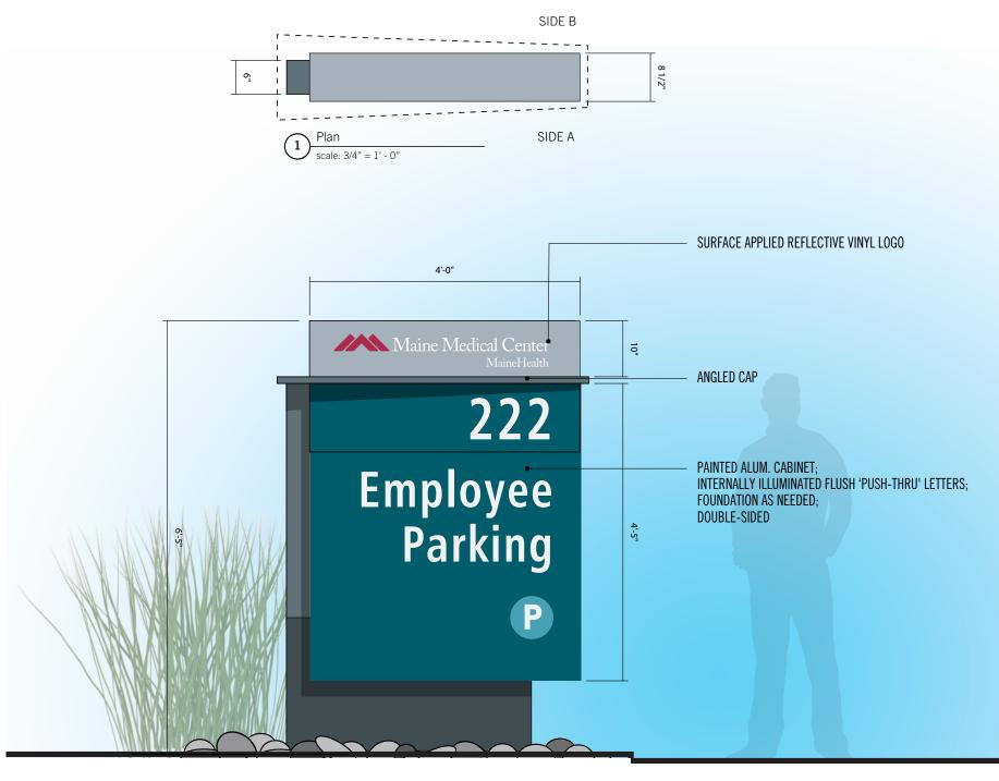
Elevation: Side A scale: 3/4" = 1' - 0"
