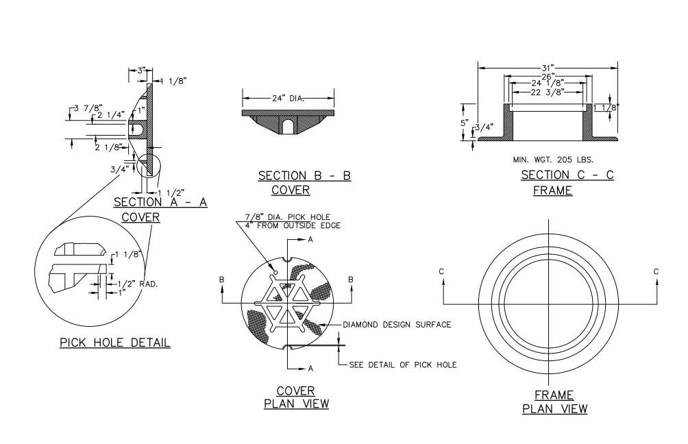
TYPICAL "A" CAST IRON MANHOLE COVER AND FRAME
