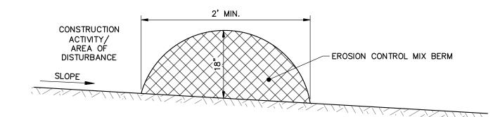
1. EROSION CONTROL MIX CAN BE MANUFACTURED ON OR OFF THE PROJECT SITE. IT MUST CONSIST PRIMARILY OF ORGANIC MATERIAL AND MAY INCLUDE: SHREDDED BARK, STUMP GRINDINGS, COMPOSTED BARK, OR ACCEPTABLE MANUFACTURED PRODUCTS. WOOD AND BARK CHIPS, GROUND CONSTRUCTION DEBRIS OR REPROCESSED WOOD PRODUCTS WILL NOT BE ACCEPTABLE AS THE ORGANIC COMPONENT OF THE MIX.
