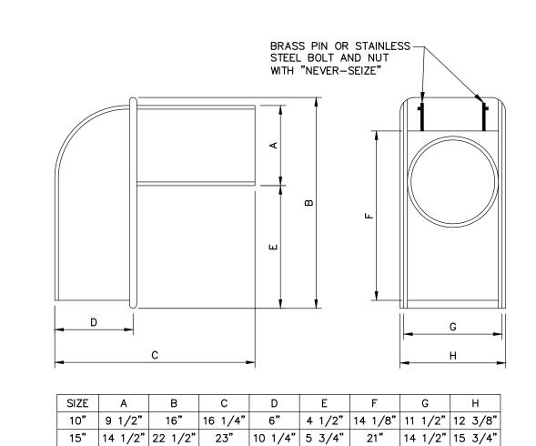
1. CASCO TRAP SHALL BE CAST IRON CASCO TRAP BY ETHERIDGE FOUNDRY OR APPROVED EQUAL.
