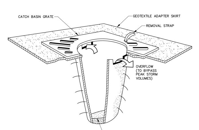
CATCH BASIN PROTECTION TO BE "SILTSACK" (BY ACF ENVIRONMENTAL) OR "STREAM GUARD" (BY FOSS ENVIRONMENTAL SERVICES). INSERT TO BE EMPTIED IN AN APPROVED MANNER WHEN IT IS 1/2 FULL OF SEDIMENT. INSPECT INSERT AFTER ALL RAINFALL EVENTS, REPAIR AND MAINTAIN
