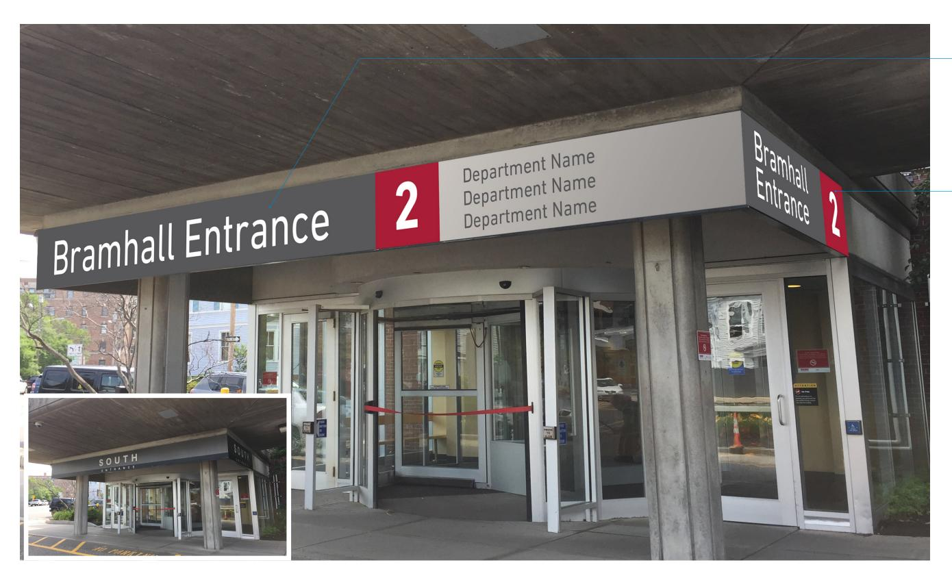
24"T x 25'-6"W x 1"D Fabricated painted aluminum panel with 1/4" painted letter forms flush mounted to panel
