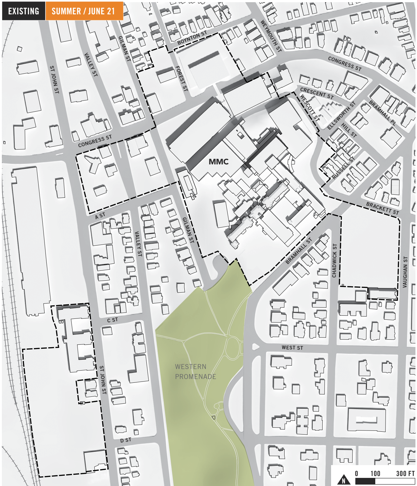
Fig.5.17 Computer-generated shadow study / Existing conditions on June 21, noon
