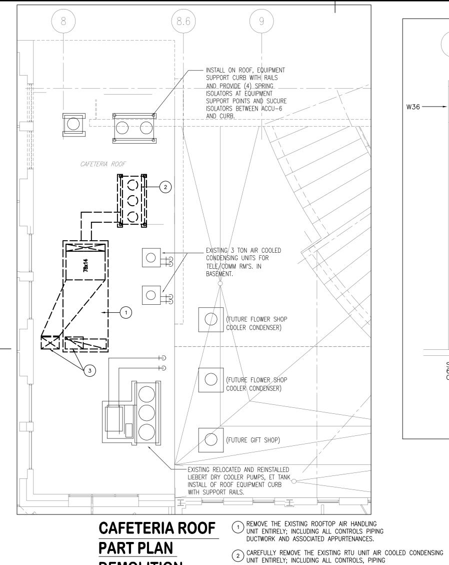
AND ASSOCIATED APPURTENANCES. RETURN CONDENSING UNIT TO OWNER AT OWNER'S (3) REMOVE EXISTING SUPPLY AND RETURN DUCTWORK ABOVE ROOF AND CUT AND CAP DUCTWORK AT ROOF LINE AND SEAL WATER TIGHT.
