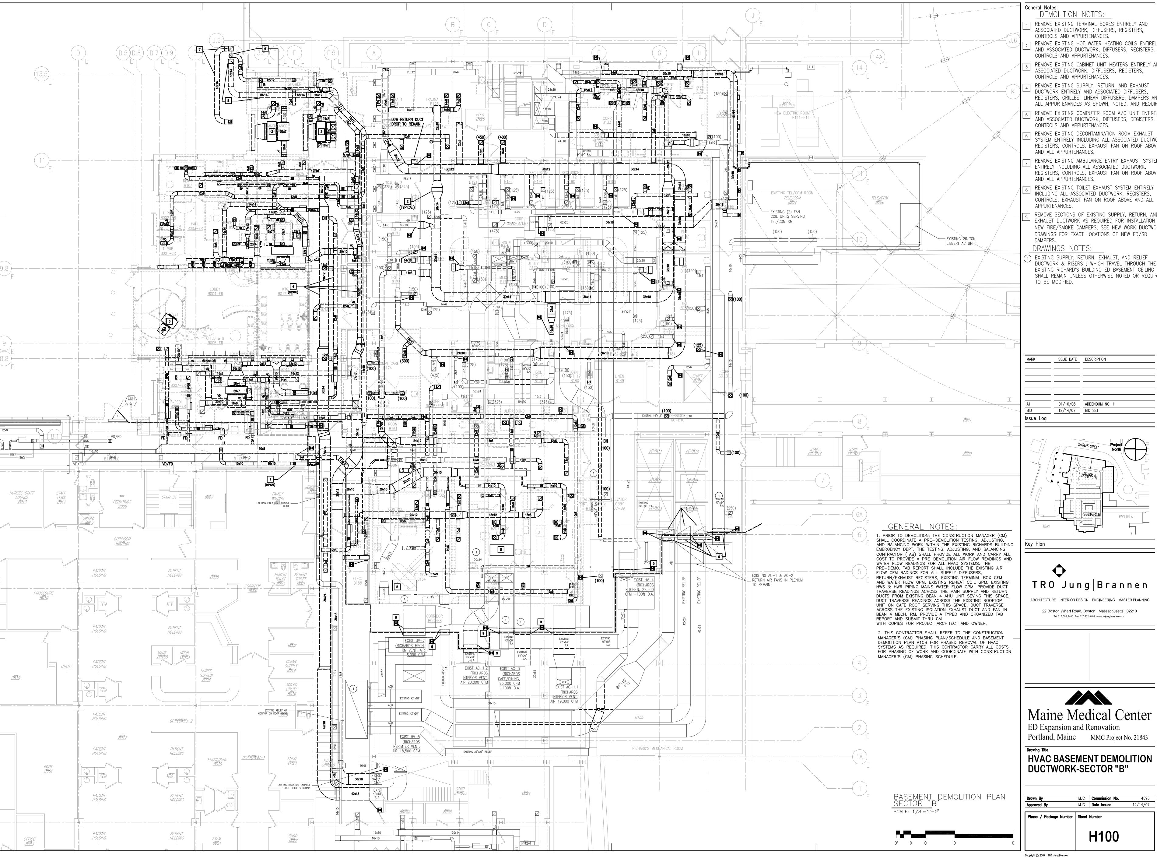
7 REMOVE EXISTING TERMINAL BOXES ENTIRELY AND ASSOCIATED DUCTWORK, DIFFUSERS, REGISTERS, CONTROLS AND APPURTENANCES.
