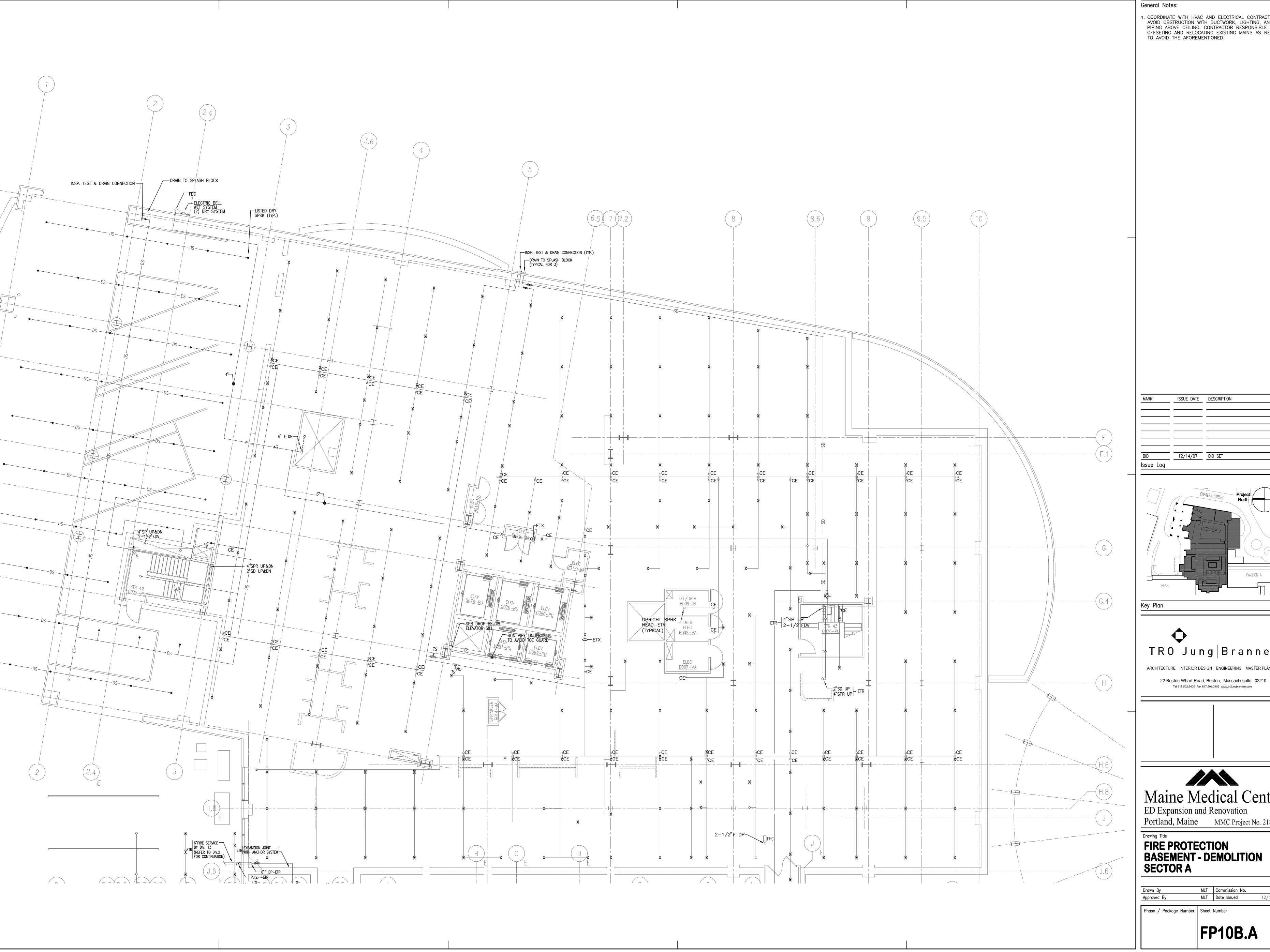
1. COORDINATE WITH HVAC AND ELECTRICAL CONTRACTOR TO AVOID OBSTRUCTION WITH DUCTWORK, LIGHTING, AND PIPING ABOVE CEILING. CONTRACTOR RESPONSIBLE FOR OFFSETING AND RELOCATING EXISTING MAINS AS REQUIRED TO AVOID THE APPRINCIPATION OF THE APPRIN
