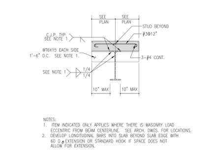
TS-19 SLAB EDGE WITH OPENINGS ON BOTH SIDES OF BEAM
