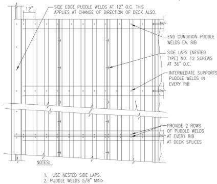
TS-12 TYPICAL FASTENING PATTERN FOR COMPOSITE METAL DECK
