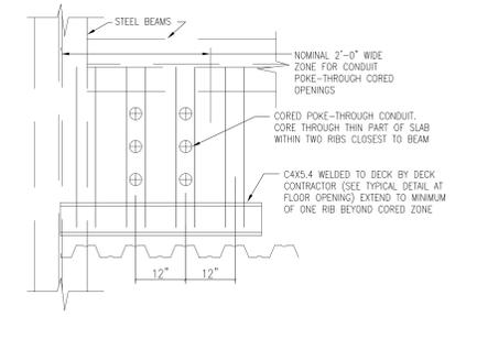
TS-14 DECK REINFORCEMENT @ ELEC./DATA/TELEPHONE ROOM CONDUIT BANK FLOOR PENETRATIONS
