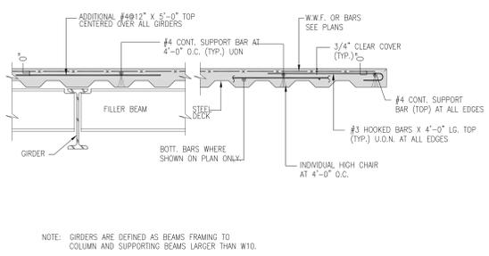
TS-15 TYPICAL COMPOSITE DECK SLAB DETAIL
