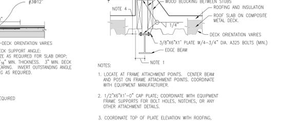
TS-25 ROOF EXHAUST SUPPORT DETAIL
