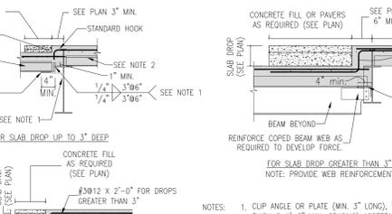
TS-24 SLAB DROP DECK AND REINFORCING DETAILS
