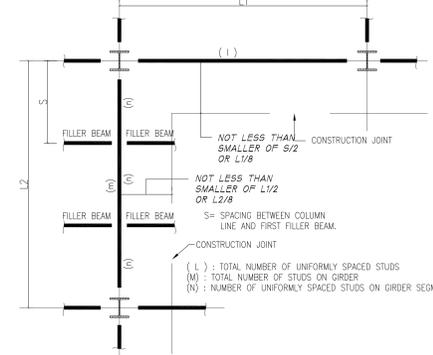
TS-18 CONSTRUCTION JOINT AND SHEAR STUD LAYOUT
