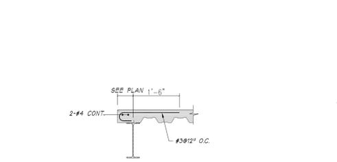
TS-21 SLAB EDGE AT FLOOR OPENING ON ONE SIDE OF BEAM
