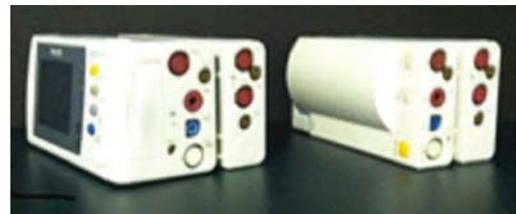
**IntelliVue Multi-Measurement Module X2 (M3002A):**
