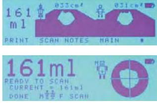
The BladderScan calculates bladder volume using patented V<sub>MODE</sub>® technology. V<sub>MODE</sub> ultrasound is easy to use and comfortable for the patient. When you press the scan button, within seconds, the V<sub>MODE</sub> technology measures ultrasonic reflections on multiple planes inside the body and produces a 3-dimensional image. Based on this image, the BladderScan calculates and displays the bladder volume.
