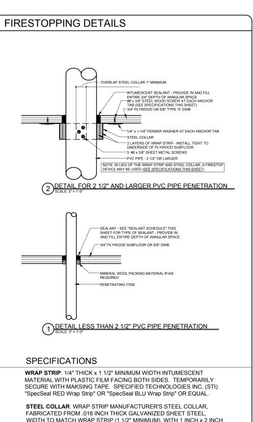
WIDTH TO MATCH WRAP STRIP (1 1/2" MINIMUM), WITH 1 INCH x 2 INCH ANCHOR TABS AND RETAINER TABS. ANCHOR TABS TO BE SYMMETRICALLY OPPOSED AROUND COLLAR; PROVIDE 3 TABS FOR 2 1/2" AND 3" PIPE; PROVIDE 4 TABS FOR 4" PIPE.
