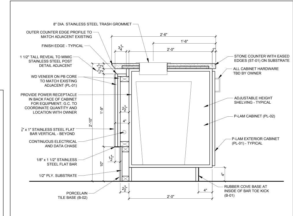
FRONT BAR TRASH RECEPTICAL SECTION DETAIL
