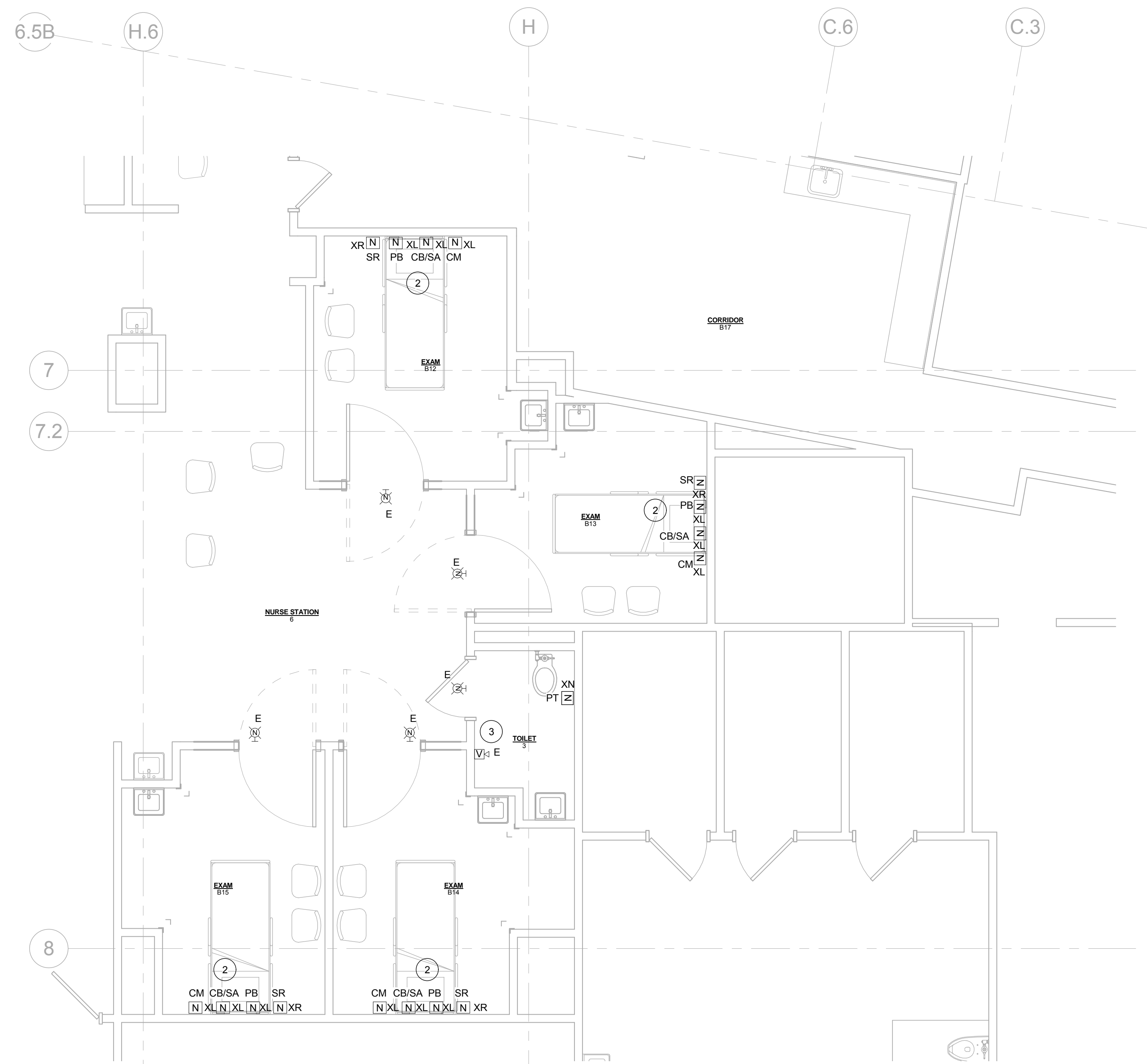
2 Electrical First Floor Signal Plan 1/4" = 1'-0"
