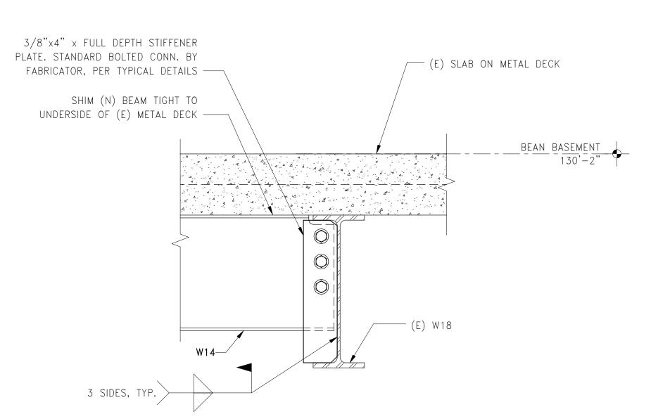
2 SECTION: (N) STEEL BEAM TO (E) BEAM AT DUMBWAITER
