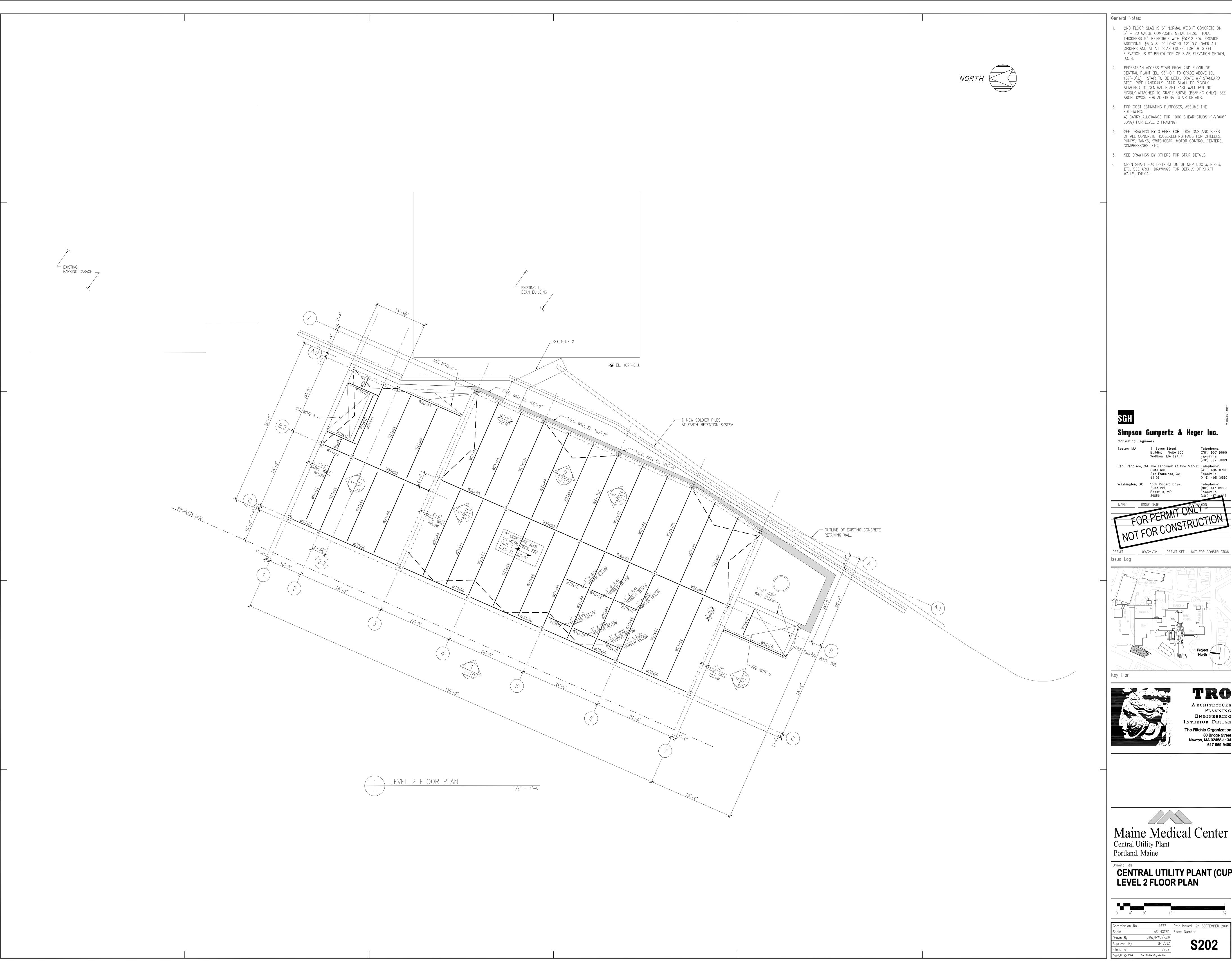
1. 2ND FLOOR SLAB IS 6" NORMAL WEIGHT CONCRETE ON 3" — 20 GAUGE COMPOSITE METAL DECK. TOTAL THICKNESS 9". REINFORCE WITH #5@12 E.W. PROVIDE ADDITIONAL #5 X 8'-0" LONG @ 12" O.C. OVER ALL GIRDERS AND AT ALL SLAB EDGES. TOP OF STEEL
