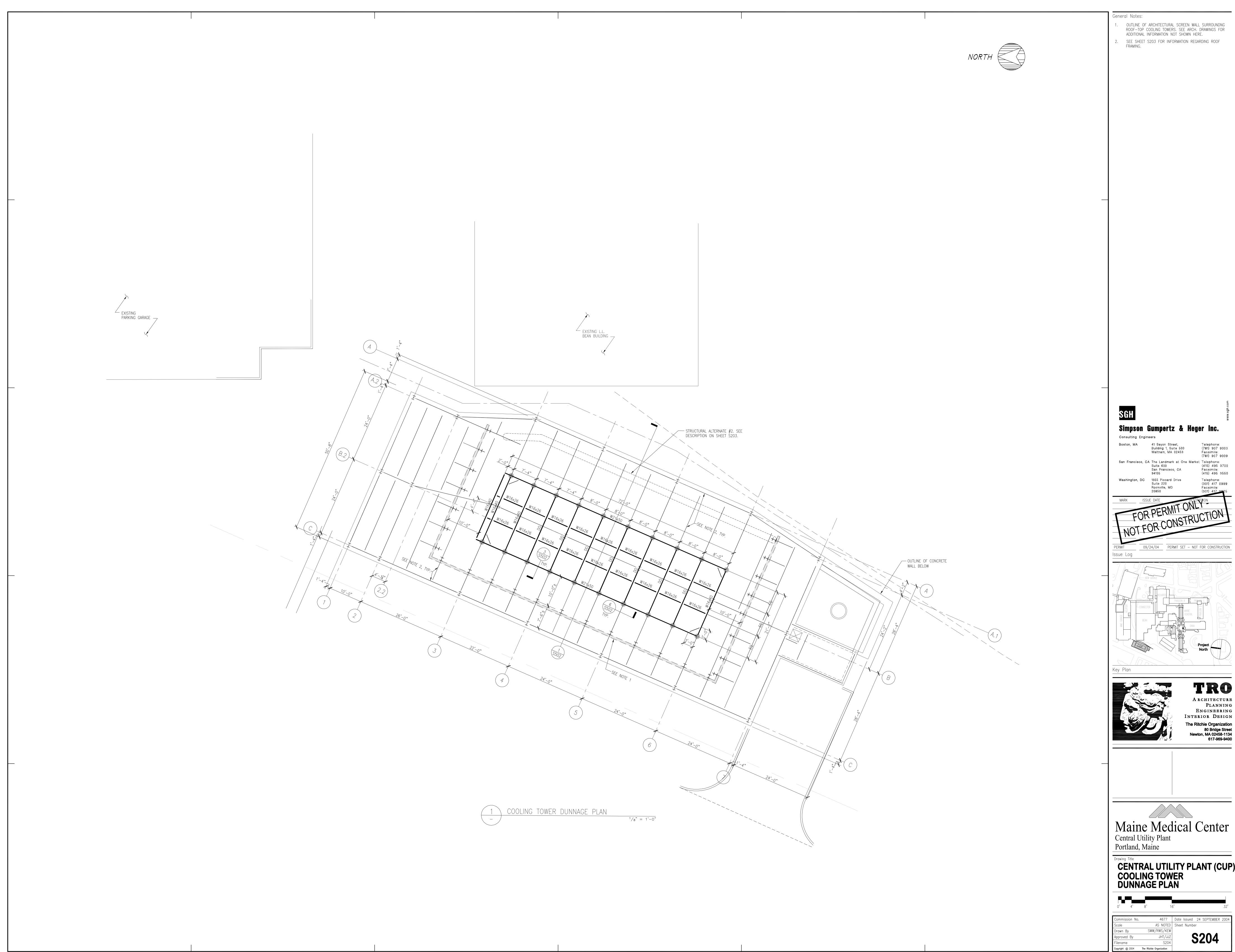
1. OUTLINE OF ARCHITECTURAL SCREEN WALL SURROUNDING ROOF-TOP COOLING TOWERS. SEE ARCH. DRAWINGS FOR ADDITIONAL INFORMATION NOT SHOWN HERE. 2. SEE SHEET S203 FOR INFORMATION REGARDING ROOF FRAMING.
