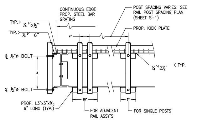
NOTE: WHERE ADJACENT RAILING ASSEMBLIES MOUNT TO STEEL PLATFORM,
