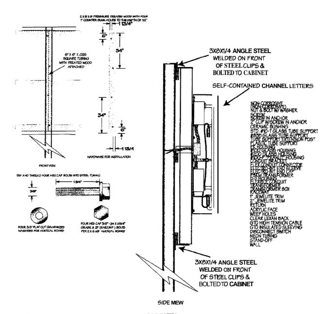
INSTALL ONE NEW 8'X 47' ALUMINUM CABINET WITH INDIVIDUAL ALUMINUM LETTERS MOUNTED TO FRONT FACE OF CABINET, LETTERS TO BE INTERANLLY ILLUMINATED WITH NEON AND COVER WITH RED & BLUE LEXAN FACES. LETTERS TO BE SELF -CONTAINED **TRANSFORMERS**
