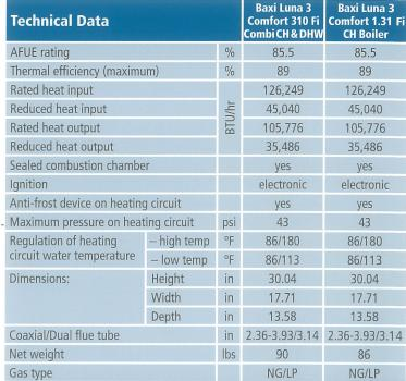
Baxi Luna 3 Comfort 310Fi is a combination central heating and DHW boiler. A separate plate-to-plate heat exchanger produces DHW of 3.3 gpm at delta T 77°F. All heat exchangers in Baxi Luna boilers are ASME H-Stamp certified, and come with a 10-year warranty.
