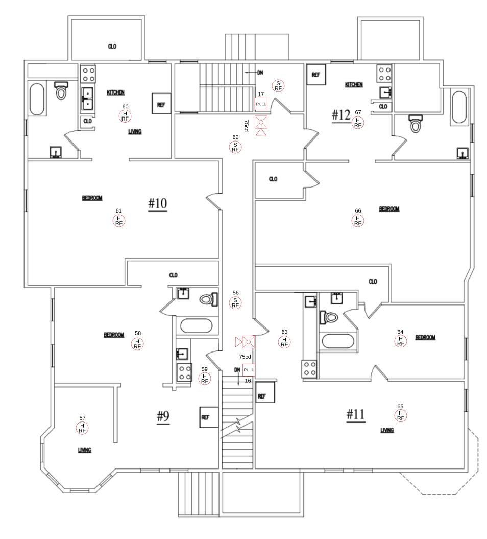
GENE A.)FIRE ALARM SYSTEM W NATIONAL ELECTRIC CODE, AF AND SHAL BE COORDINATED V JUR B.) CAUTION; DO NOT CONN PANEL(BATTERIES OR 120VAC T C.) DO NOT INSTALL FIRE ADDRESSABLE DEV D.) DO NOT INSTALL ANY AC CLOSE TO OR IN THE SAME R CON
