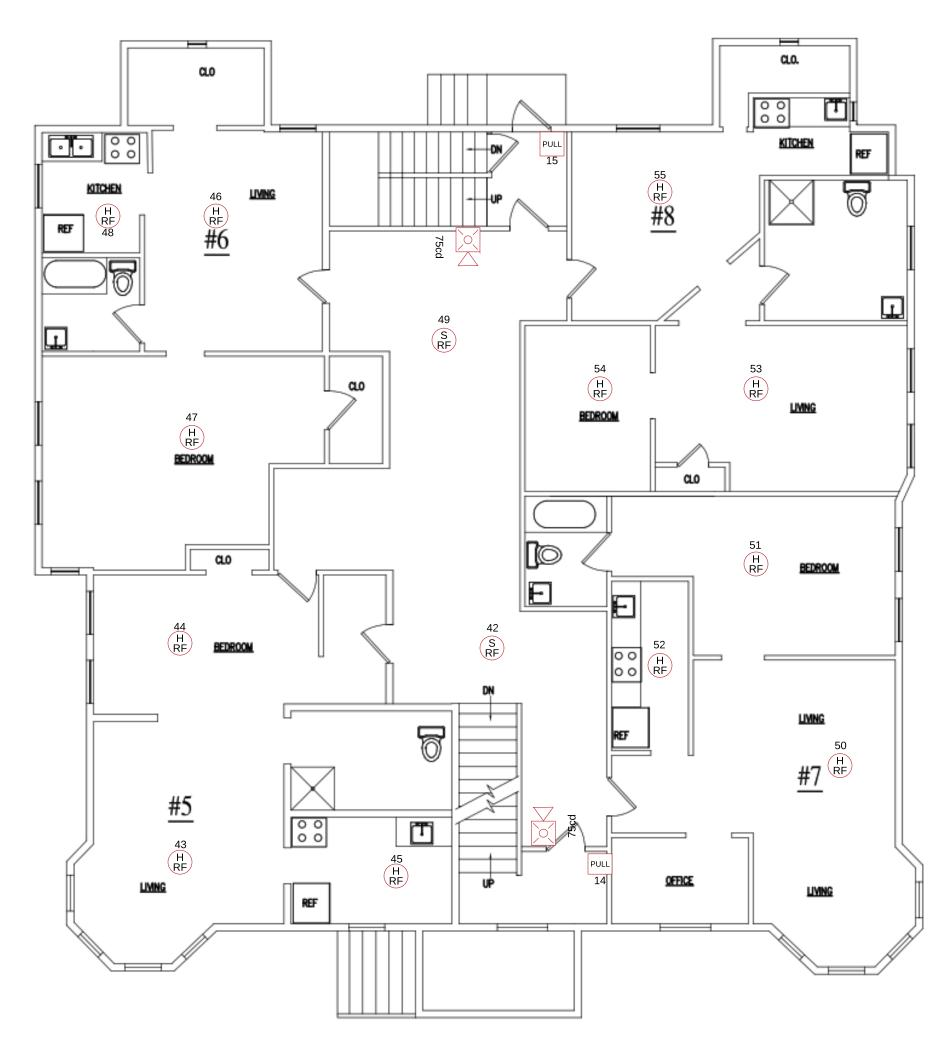
**GENERAL NOTES** A.)FIRE ALARM SYSTEM WIRING SHALL COMPLY WITH THE NATIONAL ELECTRIC CODE, APPLICABLE STATE AND LOCAL CODES AND SHAL BE COORDINATED WITH THE LOCAL AUTHORITY HAVING JURISDICTION. B.) CAUTION; DO NOT CONNECT ANY POWER TO THE CONTROL PANEL(BATTERIES OR 120VAC) UNTIL ALL FIELD WIRING HAS BEEN TESTED. C.) DO NOT INSTALL FIRE ALARM CONTROL PANEL OR ANY ADDRESSABLE DEVICES IN UNHEATED SPACE.
