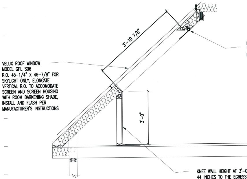
RECESS THE ROLLING SCREEN HOUSING ASSEMBLY, BY G.C.; VERIFY THE DEPTH OF THE HOUSING PRIOR TO FINAL BLOCKING LOCATION. APPROX. DEPTH OF 2-1/2".
