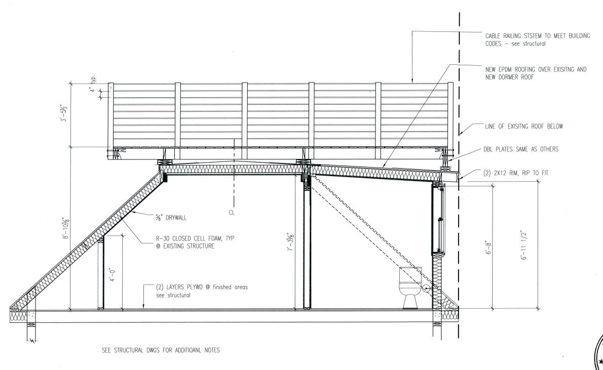
INSULATION NOTES: MIN. OF R-30 IS REQUIRED PER CODE @ ROOF. MIN. R-19 AT WALLS.
