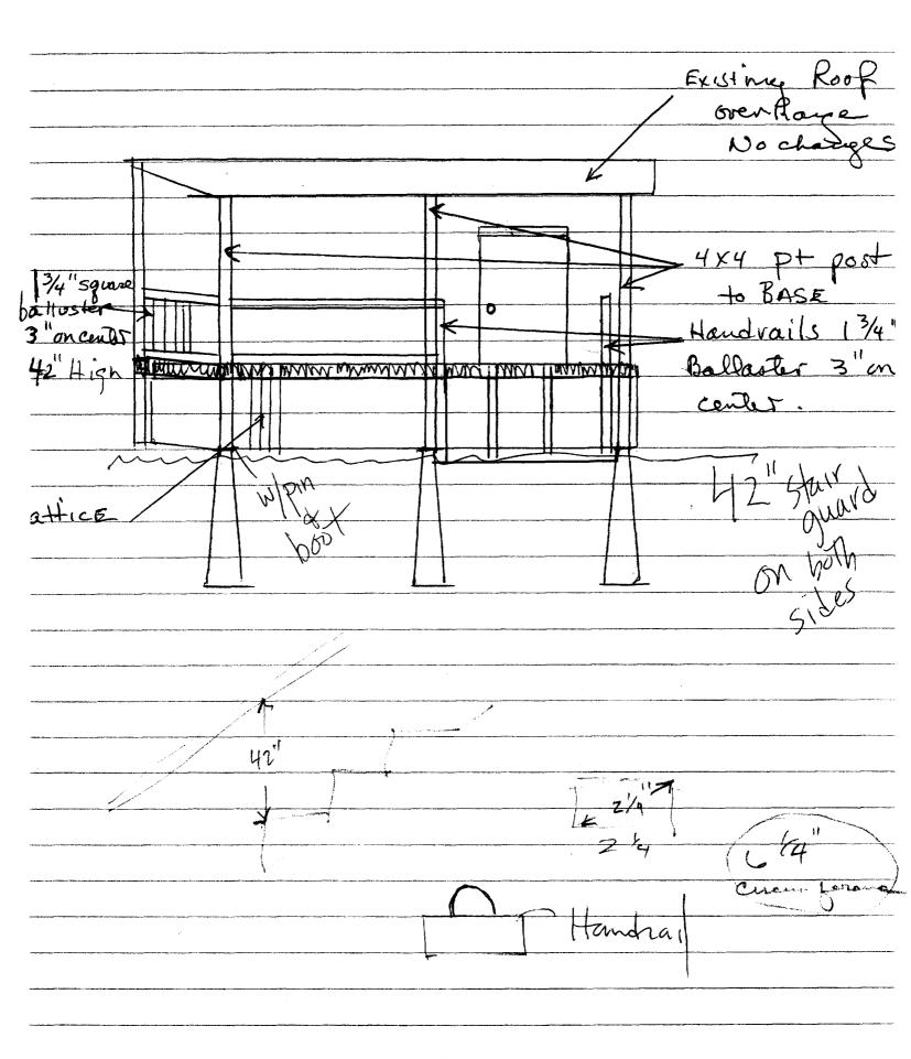
Front Entry Porch and Stairs; 115 Cherman St. Francis CloutiER Rebuild Stairs supports framing foist System and hand rails Duplicate existing MMMMM, Entry to Builting Entry to Building Buildine MM Toist Haughs Side walk 74 Decking 2x6 Legged to Building - Double Joist Double 246 Header oistnalle impers (3) 4' concrete deather Truple Jist ZX6. pilizzo Supports 2×6 Stringers 16 on center. concrete Stringer support 11" threads 7" reser set to neet code Stairs W/tapered
