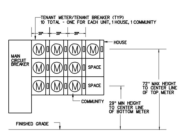
METER STACK ELEVATION BUILDING A SCALE: NONE
