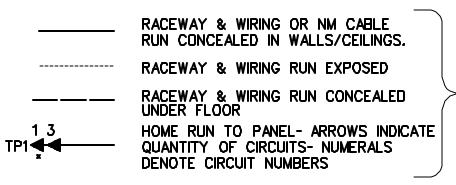
BRANCH CIRCUIT WIRING SHALL CONSIST OF 2+12, 1+12G, 1/2 "C UNLESS OTHERWISE NOTED. ASTERISK INDICATES +10 AWG FOR ALL CIRCUITS CONTAINED IN HOMERUN.
