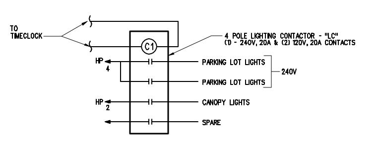
LIGHTING CONTACTOR "LCA" DETAIL SCALE: NONE
