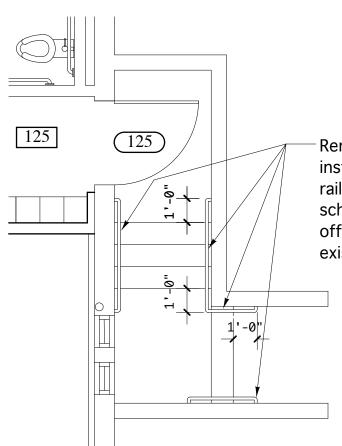
Remove exist'g handrails and install new painted galv. steel rails consisting of 1 1/2" O.D. schedule 40 pipe. Set rail at 34" off of nosings and attach to existing brick walls
