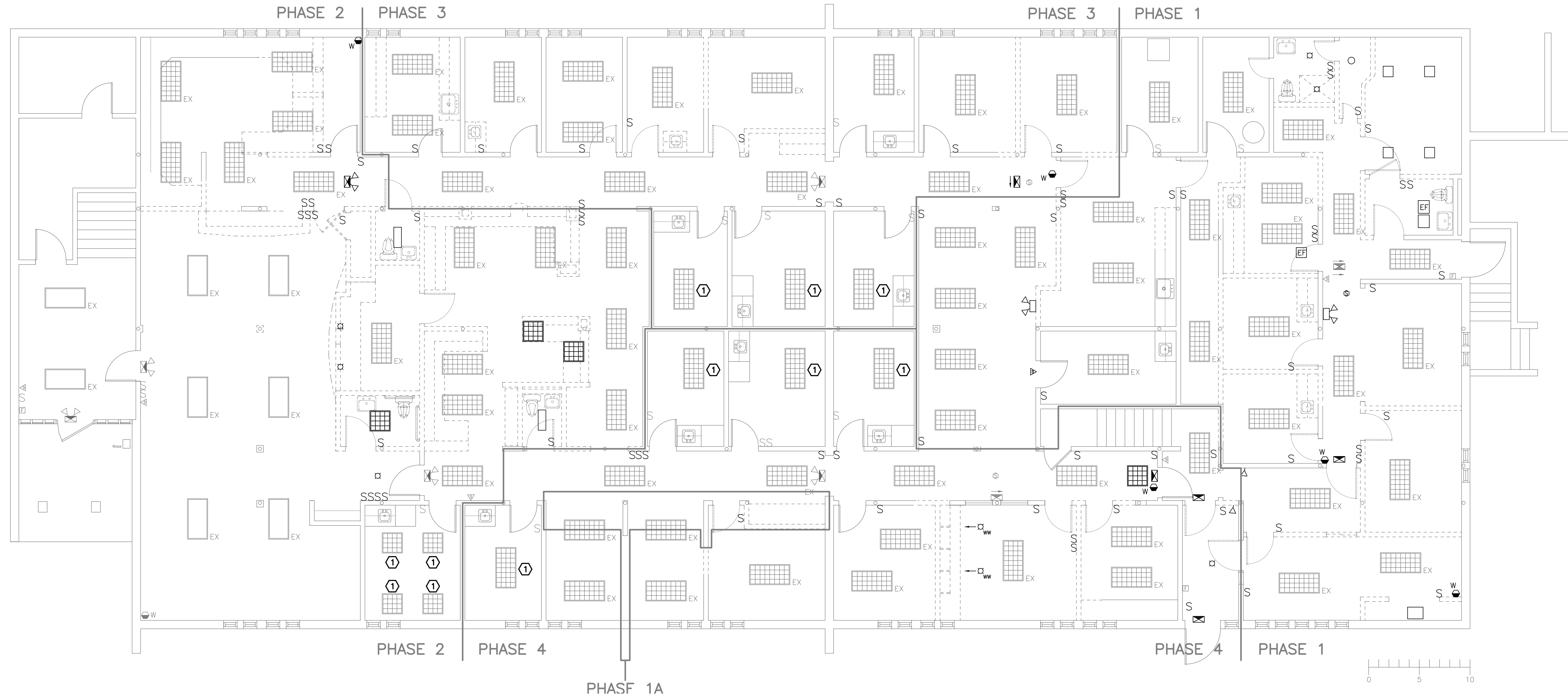
① ELECTRICAL LIGHTING DEMOLITION PLAN SCALE: 3/16" = 1'-0"
