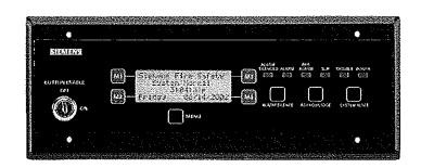
The Model FS-RD2 Remote Display is used for annunciating system events remotely from the fire alarm control panel on the FireSeeker FS-250 system. The FS-RD2 will mimic the system status LEDs and the 80-character event message found on the main system panel. The 4 x 20 LCD backlit display will illuminate upon receiving any event from the system, or upon pressing any button on the FS-RD2.
