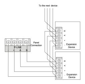
RA-6500F Class A Wiring Example Fig 2
