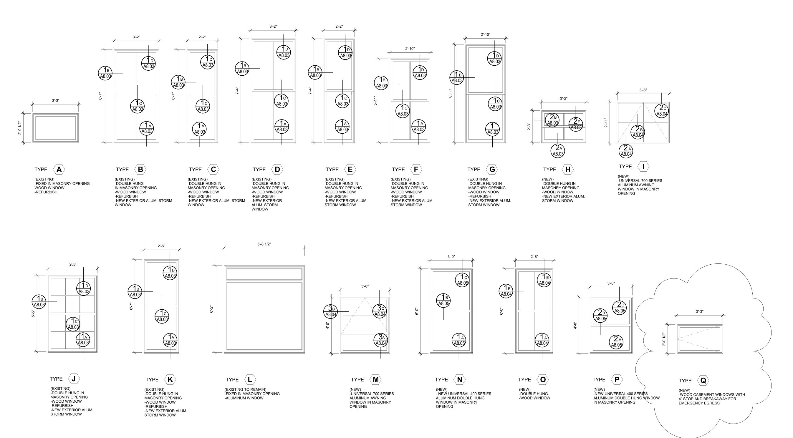
PROVIDE SILL LOCKING MECHANISM AT ALL OPERABLE WINDOWS - REFERENCE SPECIFICATION PROVIDE SCREENS AT ALL STORM WINDOWS INSPECT AND REPAIR/REPLACE WINDOW PAN FLASHING WITH LIKE MATERIALS. PROVIDE NEW METAL FLASHING AT NEW WINDOWS.
