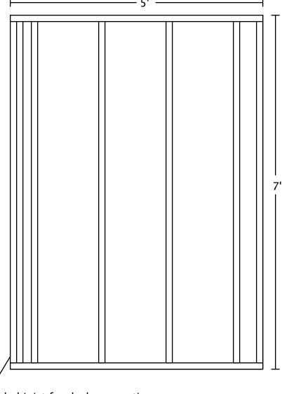
2X10 joists for added height to accommodate deck connection and match existing kitchen floor height
