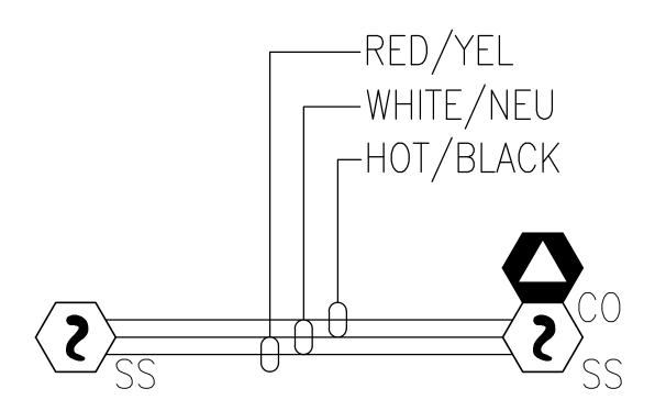
ROOM DETECTOR CONNECTION DIAGRAM (TYPICAL)
