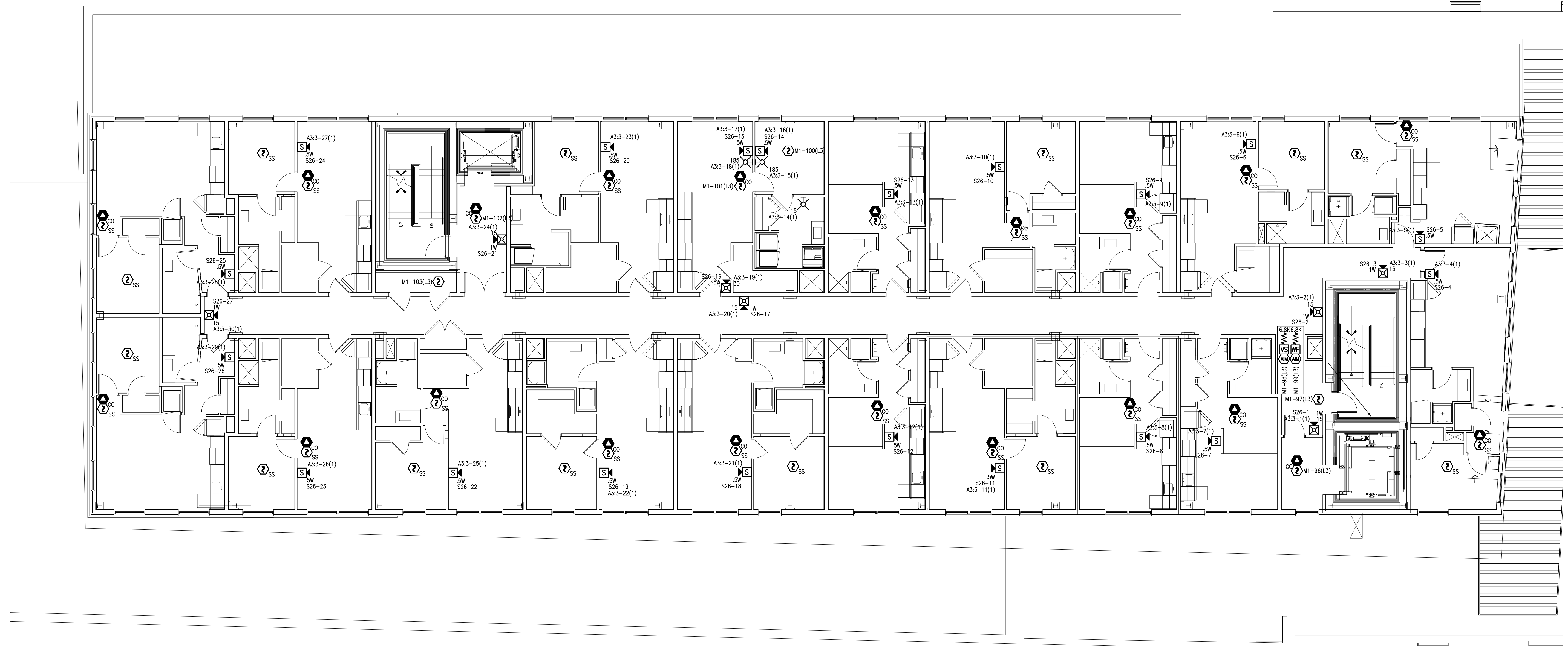
PLAN NORTH DEVICE PLACEMENT PLAN - SEVENTH FLOOR SCALE: 1/8" = 1'-0" 0 4 8 16 (IN FEET)
