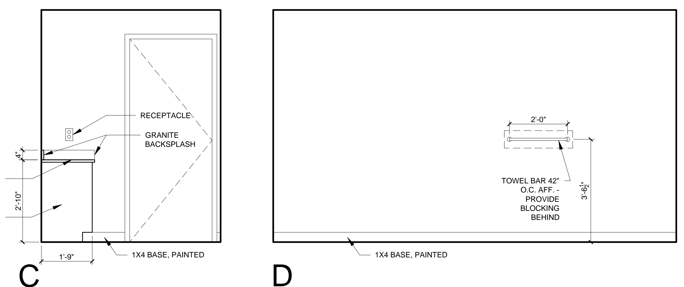
3 UNIT 320-620 INTERIOR ELEVATIONS CONTINUED 1/2" = 1'-0"
