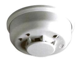
Honeywell's 5806W3 is a 3V battery operated, photoelectronic smoke detector with a built-in wireless transmitter. It facilitates fire verification for false alarm reduction requirements by ANSI/SIA CP-01standards and is intended for use with any of Honeywell's 5800 Series wireless receiver/transceivers for residential installations. The 5881ENHC or 5883H receivers are required for commercial installations.
