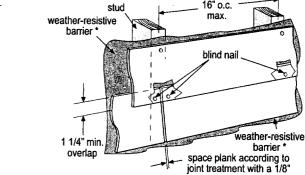
Hardiplank siding cannot be blind nailed 24" o.c. 12" wide Hardiplank siding cannot be blind nailed. When blind nailing 9 1/4" or 9 1/2" Hardiplank, use 11 ga. roofing nail x 1 1/4" long.
