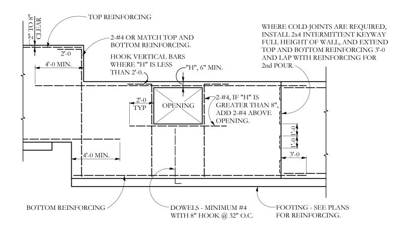
TYPICAL REINFORCING AT STEPS AND OPENINGS
