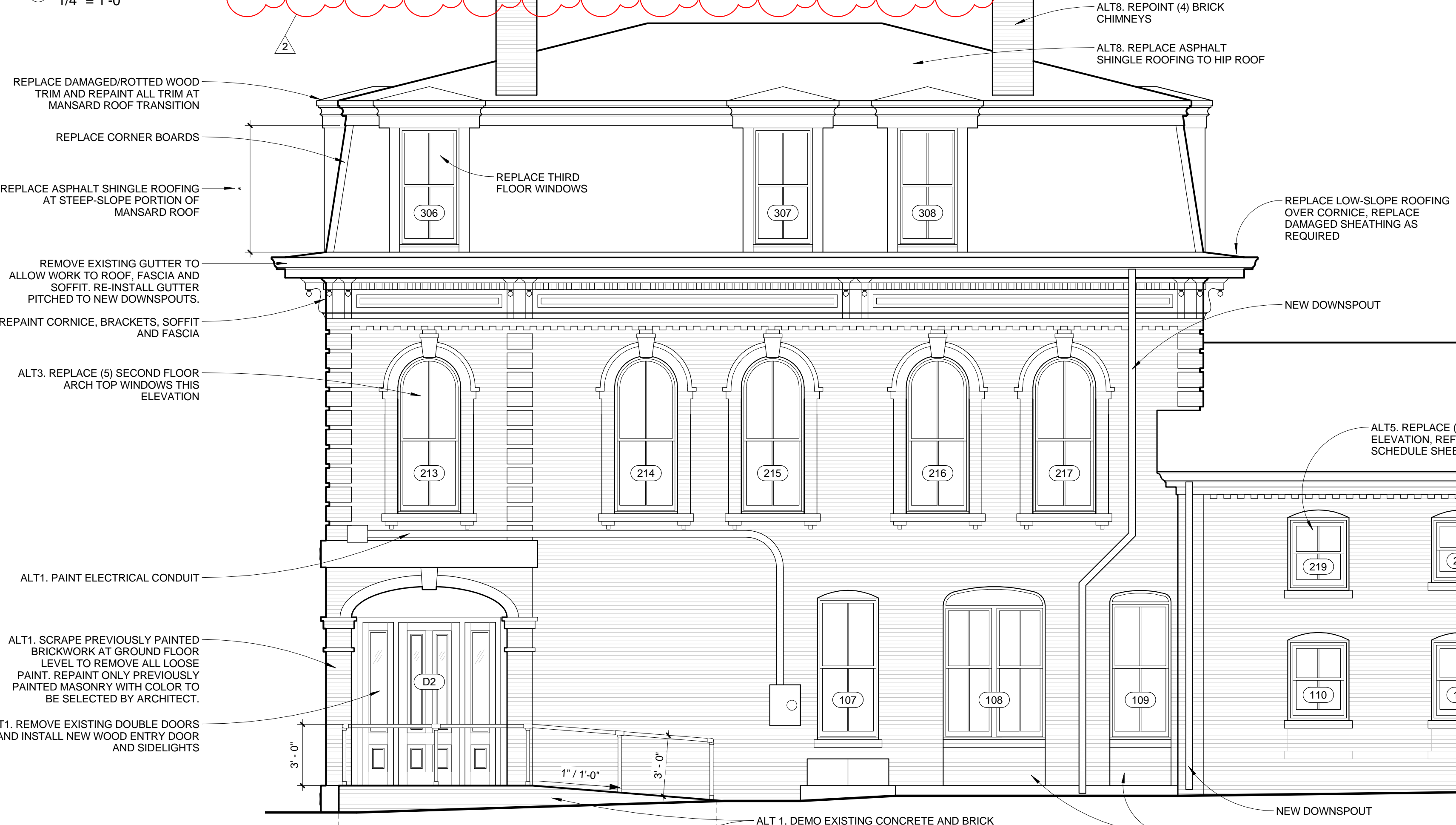
3 SOUTH ELEVATION 1/4" = 1'-0" ALT 1. DEMO EXISTING CONCRETE AND BRICK ENTRY RAMP. INSTALL NEW POURED CONCRETE FROST WALLS AND FOOTINGS. NEW CONCRETE RAMP AT 1:12 PITCH WITH LEVEL LANDING AT TOP AND BOTTOM. FACE CONCRETE FROST WALLS AND RAMP SURFACE WITH BRICK PAVERS. INSTALL NEW PAINTED METAL PIPE RAIL. ALT 7. REMOVE WINDOWS AND WOOD FRAMED INFILL AT ORIGINAL DOOR OPENINGS. INSTALL NEW WINDOWS WITH BRICK SILLS AND BRICK WALL INFILL BELOW - SET BACK NEW BRICK 1/2" FROM FACE OF ADJACENT BRICK
