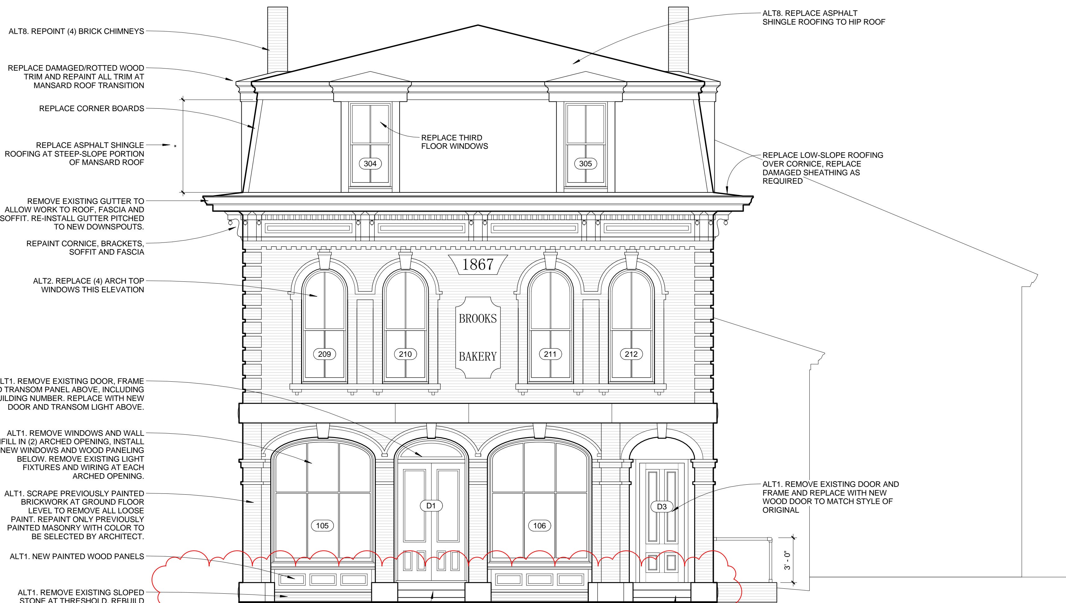
1 WEST ELEVATION - STREETFRONT 1/4" = 1'-0" (2) NEW GRANITE STEPS, LENGTH TO FIT BETWEEN EXISTING GRANITE PIER BASES. EACH STEP TO HAVE 10" CLEAR RUN AND 6" +/- RISE. VERIFY HEIGHT IN FIELD TO CREATE (3) EQUAL RISERS BETWEEN SIDEWALK AND EXISTING GRANITE TOP STEP. SET ON NEW CONCRETE PAD. NEW METAL PIPE RAIL ONE SIDE ONLY (2) NEW GRANITE STEPS, LENGTH TO FIT BETWEEN EXISTING GRANITE PIER BASES. EACH STEP TO HAVE 10" CLEAR RUN AND 6" +/- RISE. VERIFY HEIGHT IN FIELD TO CREATE (3) EQUAL RISERS BETWEEN SIDEWALK AND EXISTING GRANITE TOP STEP. SET ON NEW CONCRETE PAD. NEW METAL PIPE RAIL BOTH SIDES
