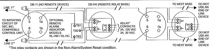
\*\*HFP-11/HFPT-11/HFPO-11SFP-11/SFPT-11/SFPO-11 is a polarity insensitive detector. Line 1 and Line 2 can be either line of the loop.
