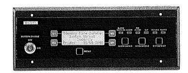
The Model FS-RD2 Remote Display is used for annunciating system events remotely from the fire alarm control panel on the FireSeeker FS-250 system. The FS-RD2 will mimic the system status LEDs and the 80-character event message found on the main system panel. The  $4 \times 20$  LCD backlit display will illuminate upon receiving any event from the system, or upon pressing any button on the FS-RD2.
