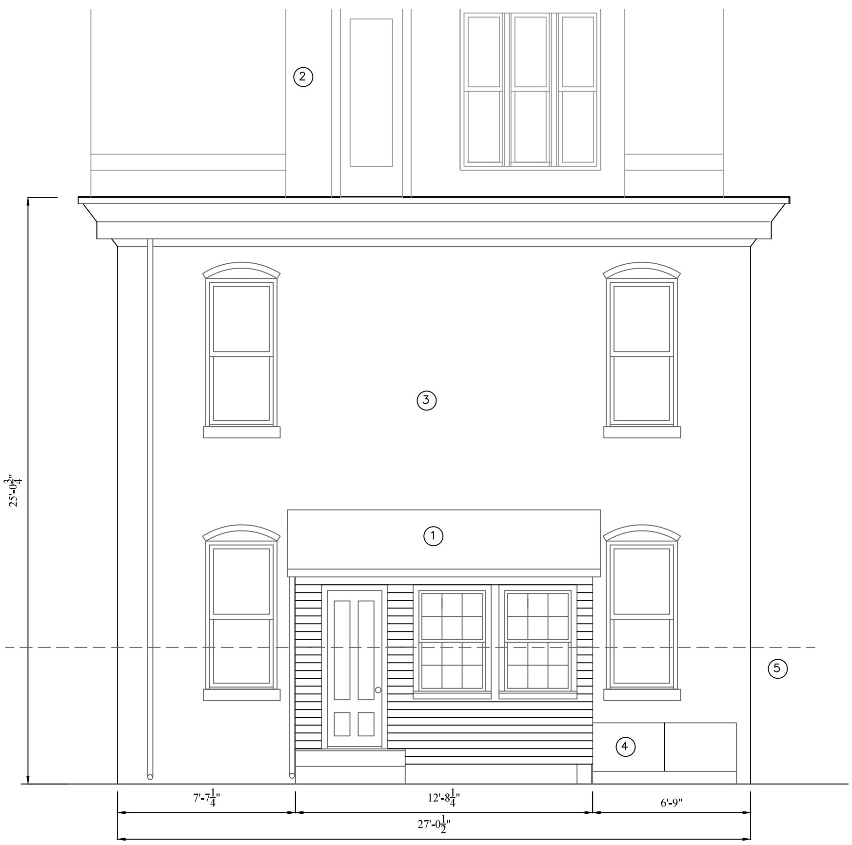
1 EXISTING BUILDING REAR (WEST) ELEVATION SCALE: 1/4" = 1'-0"
