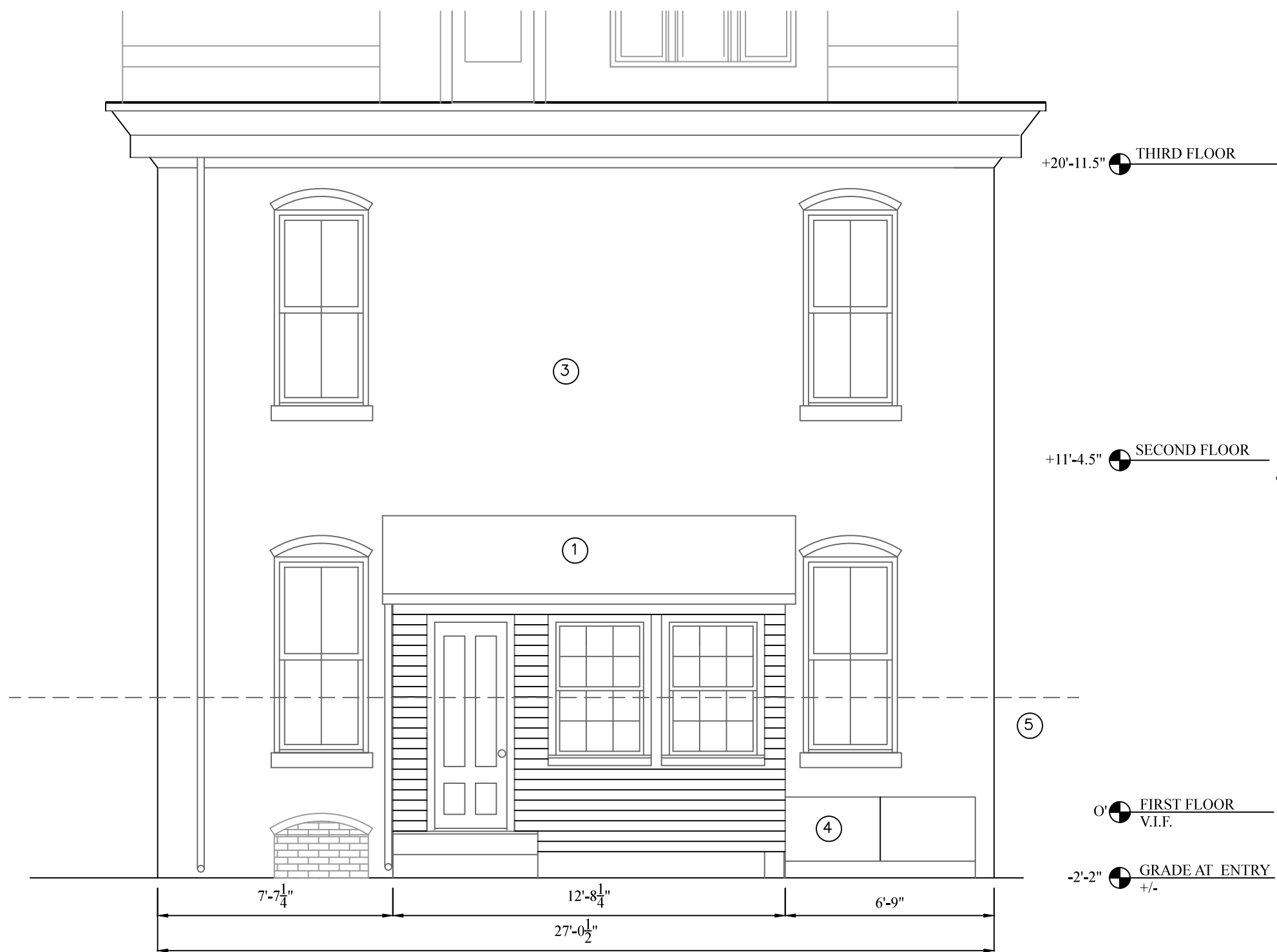
3 EXISTING AND PROPOSED ENTRY SIDE ELEVATIONS SCALE: 1/4" = 1'-0"
