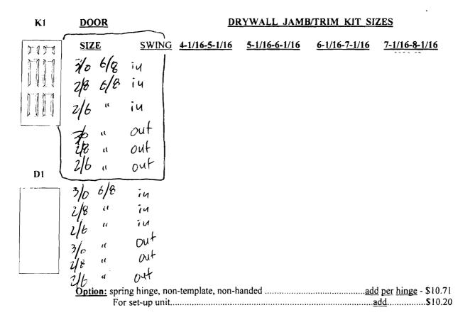
To Determine Rough Opening: Add 1" to the width and 1-1/4" to the height of the nominal door dimension
